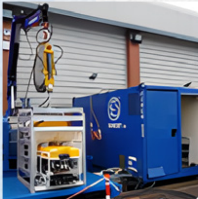
SAAB SEAEYE TIGER ROV WITH 4 FUNCTION HYDRAULIC MANIPULATOR, LARS AND CONTROL CABIN
